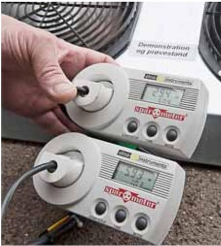
Measurements show an 80% difference in energy consumption between a Q and an iQ motor.
